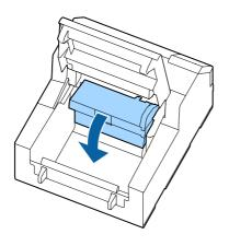
6 Attach adhesive side of a label to the roller, and peel it off slowly. Repeat this action until paper dust or adhesive is completely removed from side to side of the roller. If some labels have stuck on the roller, carefully remove them as they can cause a paper jam.
