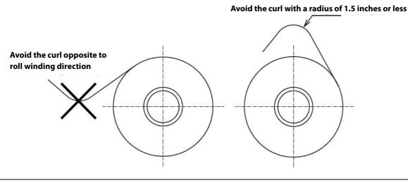
The outer diameter of the roll core should be at least 82 mm.
