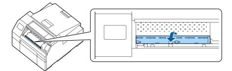
**5** Use a cloth or cotton swab to remove adhesive adhered to the platen.
