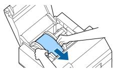
**10** Rotate the spindle to remove looseness in the paper.
