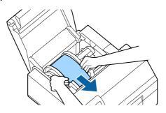
**1 O** Rotate the spindle to remove looseness in the paper.
