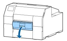
Cut the paper near the paper ejection slot. 2
