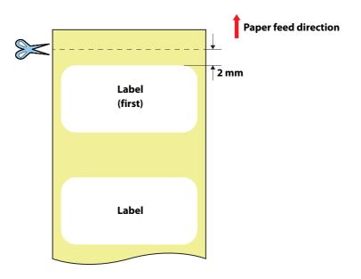
2 On the operation panel of the printer, select [Not Feed] from [Actions when Replacing Media].
